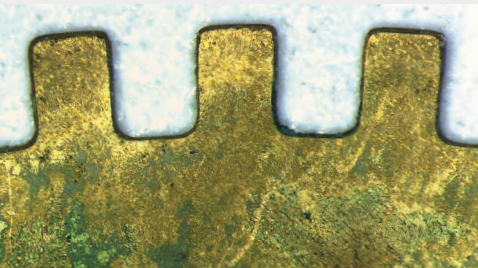
Oxidation on gear wheel
