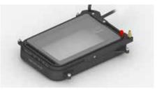
**020**Okolab stage top incubator for Leica Super Z Galvo Stage
