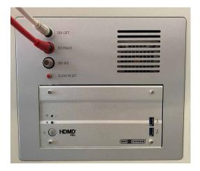
► Connect the 2 SDI cables of the heads-up monitor to the GLOW800 faceplate of M530 OHX.
