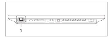
Press the on/off switch (1) on the bottom side of the heads-up monitor to switch it on.
