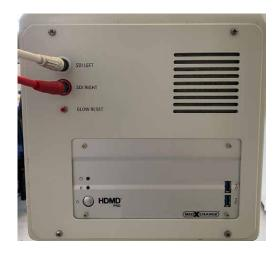
Connect the 2 SDI cables of the heads-up monitor to M530 0H6 or ARveo.
