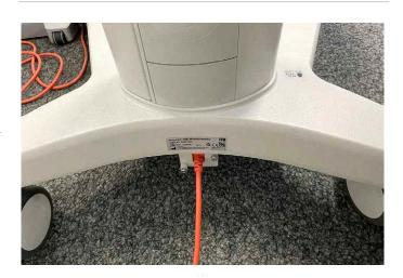
Connect the cable of the power socket at the bottom of the cart to the power outlet.
