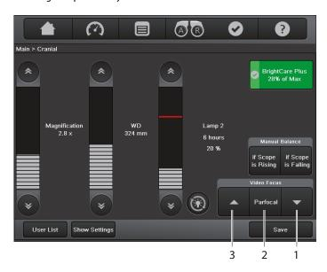
► The video focus can be adapted to your needs by pressing the focus button up (3) or/and down (1). This command can be given to the GUI and from the handle, if defined.
