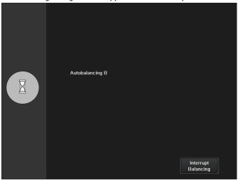
Balancing is completed when the acoustic signal no longer sounds and the autobalancing push-button is no longer flashing.
