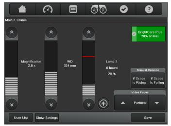
Microscope is too heavy touch "if Scope is Falling" key
