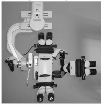
► Move the B axis with switch (3) until the optics carrier is balanced.
