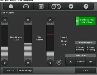
When BrightCare Plus is activated, the red line on the brightness adjustment bar shows the maximum adjustable brightness for the current working distance.
