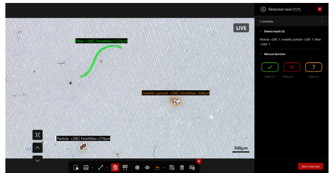
Example of analysis of particles and fibers on a sample with Aivaro AI Feature Detection.
