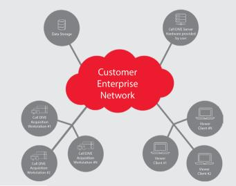
Cell DIVE Connect allows a user to share a database of slides and metadata between multiple Cell DIVE Imagers and their Acquisition Workstations. A basic diagram of the deployment is shown above.
