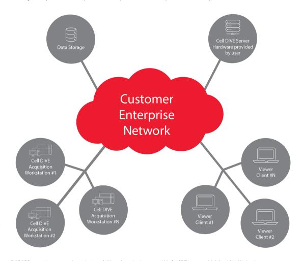
Cell DIVE Connect allows a user to share a database of slides and metadata between multiple Cell DIVE Imagers and their Acquisition Workstations. A basic diagram of the deployment is shown above.
