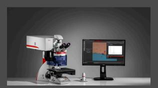
**Laser induced breakdown spectroscopy** (LIBS) enables simultaneous visual and chemical analysis. The DM6 M LIBS 2-in-1 solution allows fast particle identification:
