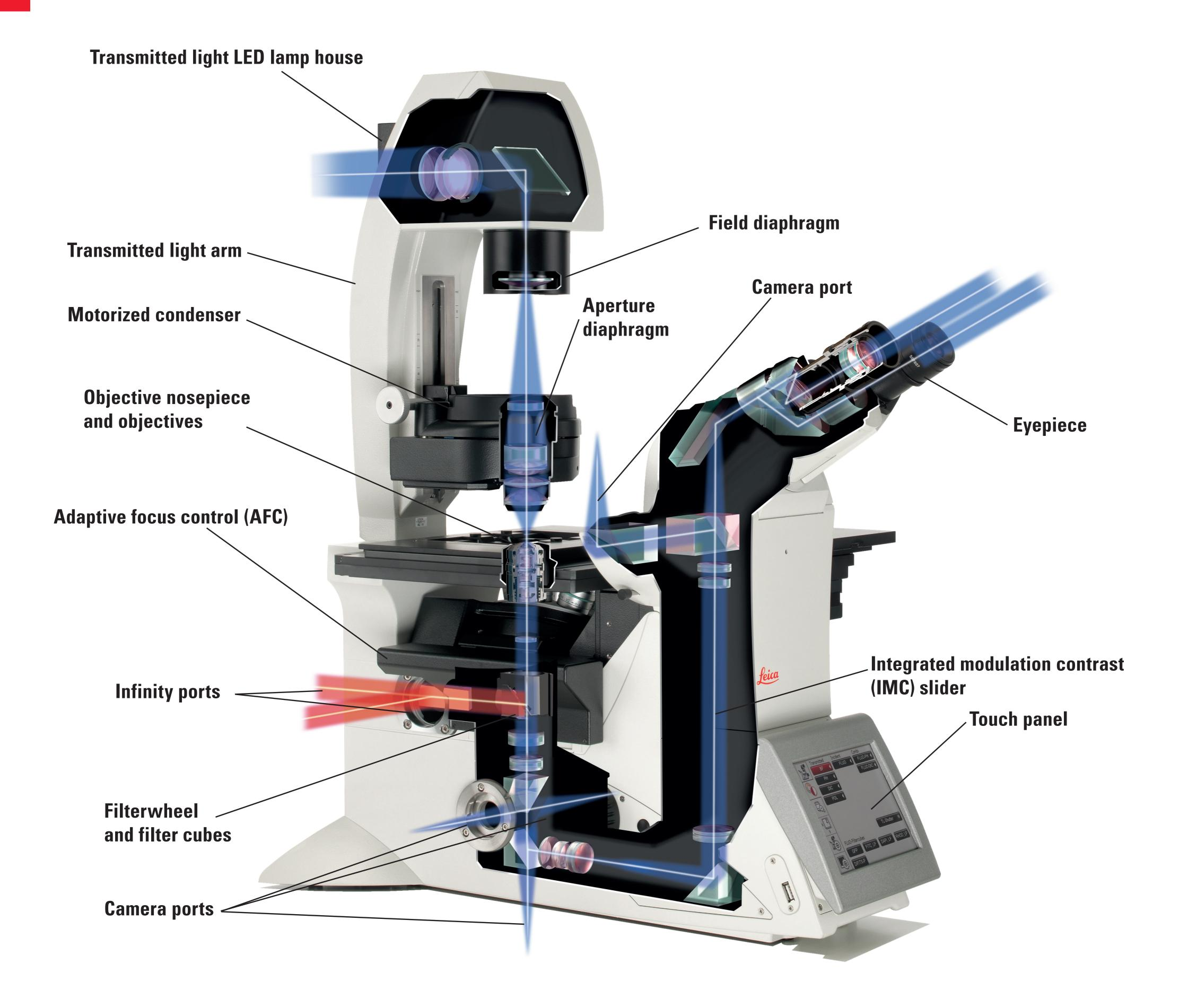
Innovation from every perspective – Inverted microscope platform DMi8 with Infinity Ports from Leica Microsystems
