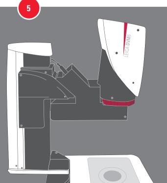
Mount zoom module on interface module repeating the procedure backwards:
