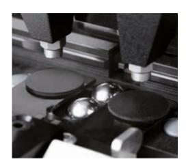
The technique of producing a straight, controlled break in a strip of scientific-quality glass requires that the knife maker apply equal weight and pressure to each side of the score. In addition, the support elements that touch the glass from below must have minimum surface contact to avoid uncontrolled stress applied to the glass prior to the break.
