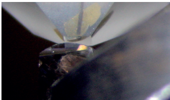
Diamond miller Si sample trimming
