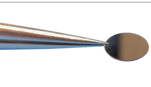
Even hard and brittle materials can be thinned to be prepared for TEM investigation e.g. for ion thinning with the
