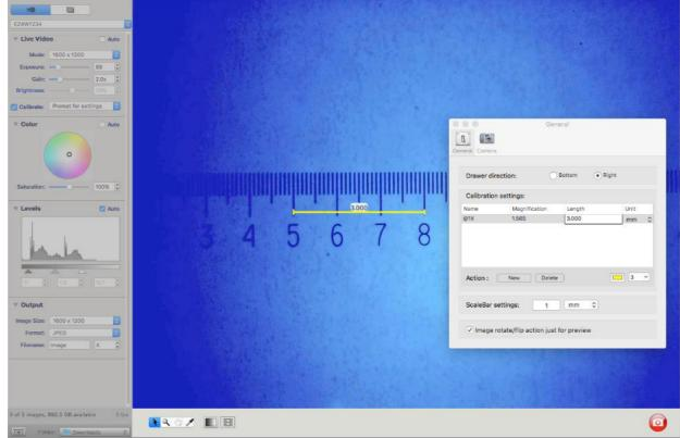
Drag the line to match the desire position, input the correct value for length (3mm in this example)
