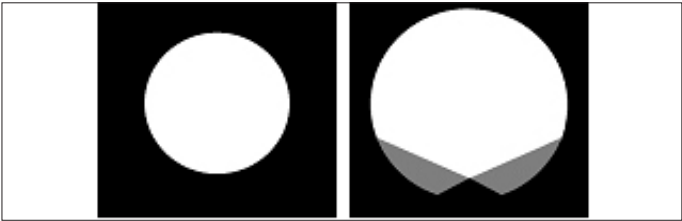
Illumination pattern sketches for circular (left) and bar (right) glare masks. The gray areas in the bar sketch denote areas that receive 50% illumination.
