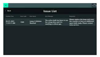
Check the life time of the bulb(s) and replace the bulb(s) if the efficiency is too low.
