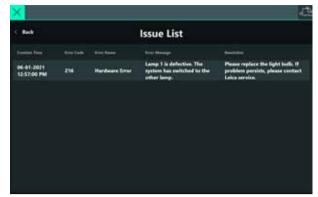
Exchange the defective bulb with a new one before your next case.
