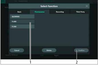
► Select the desired function (1) and apply with Confirm (2). The selected function is displayed in the selection field. The selections are identical to those for the handles with the exception of the brakes.
