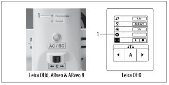
The following LEDs on the swing arm are significant for the Leica FL400 for M530 application:
