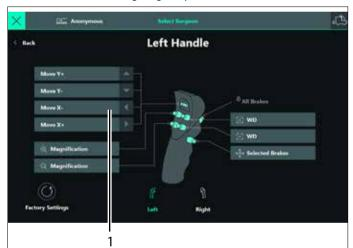
When you are on the handle configuration page, press the button you want to assign for the activation of the Leica FL400. In this example we select the left button of the joystick (1). The "Select function" popup window for the selected button appears:
