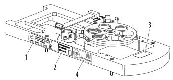
The type label is located on the side of the Leica FL400 for M530 filter module.
