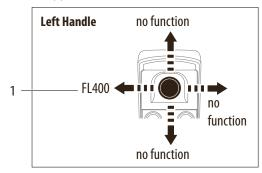
Press the joystick to the left: The main page for "Fluorescence FL400" with the actual settings in Fluorescence FL400 mode are displayed:
