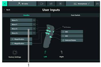
► When you are on the handle configuration page, press the button you want to assign for the activation of the Leica FL400. In this example we select the left button of the joystick (1).
