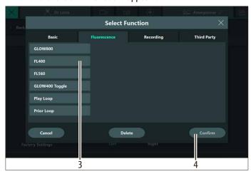
► Select the Leica FL400 function (3) and press "Confirm" (4) to save the settings.
