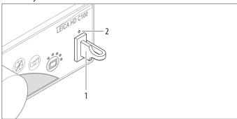
Take off the USB port protective cap (1) on the front side of the control unit and insert the USB storage device.
