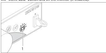
Press the "Scene data" button (1) until the LED for the desired scene data lights up on the control unit.
