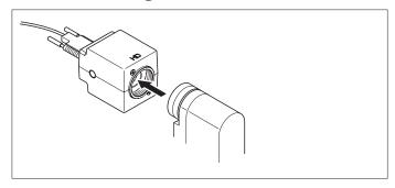
The camera C-mount interface is screwed on to the C-mount interface of the video adapter.
