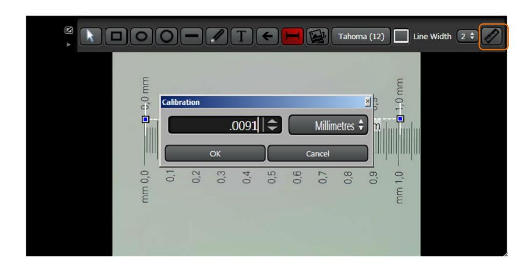
Click the Calibration icon and input the calibration factor. For decimals, start with a "0" before the decimal point. Then select units of measure and click "OK".
