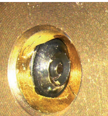
Leica LED5000 NVI: internal image of a grub screw in a brass gear wheel
