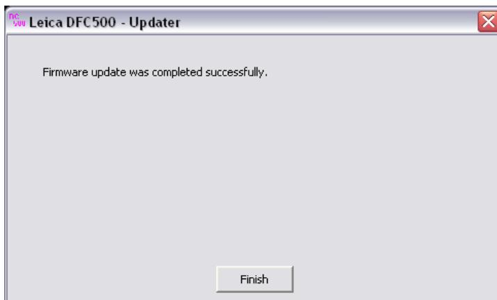
Wait until the *Finished* button is active before using or disconnecting the camera.
