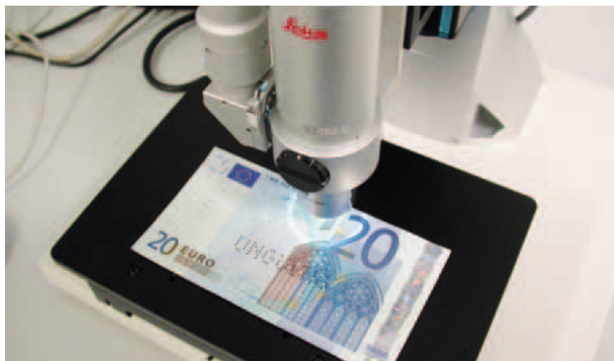
Fig. 2: Analyzing a banknote with the Leica DVM5000: with the instrument's high magnification levels, versatile zoom optics, and large depth of field, experts can discover how counterfeit money was produced and match a forgery to a known "trademark."
