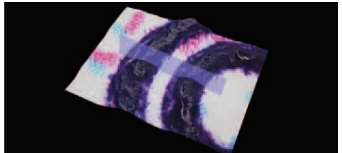
Fig. 6: 3D image capture of the intaglio printing on a genuine 500 euro bill. A section was made through the profile.
