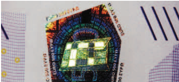
Fig. 3: Foil element of the 500 euro note, image acquired with the digital microscope's swing stand at a 45° angle.
