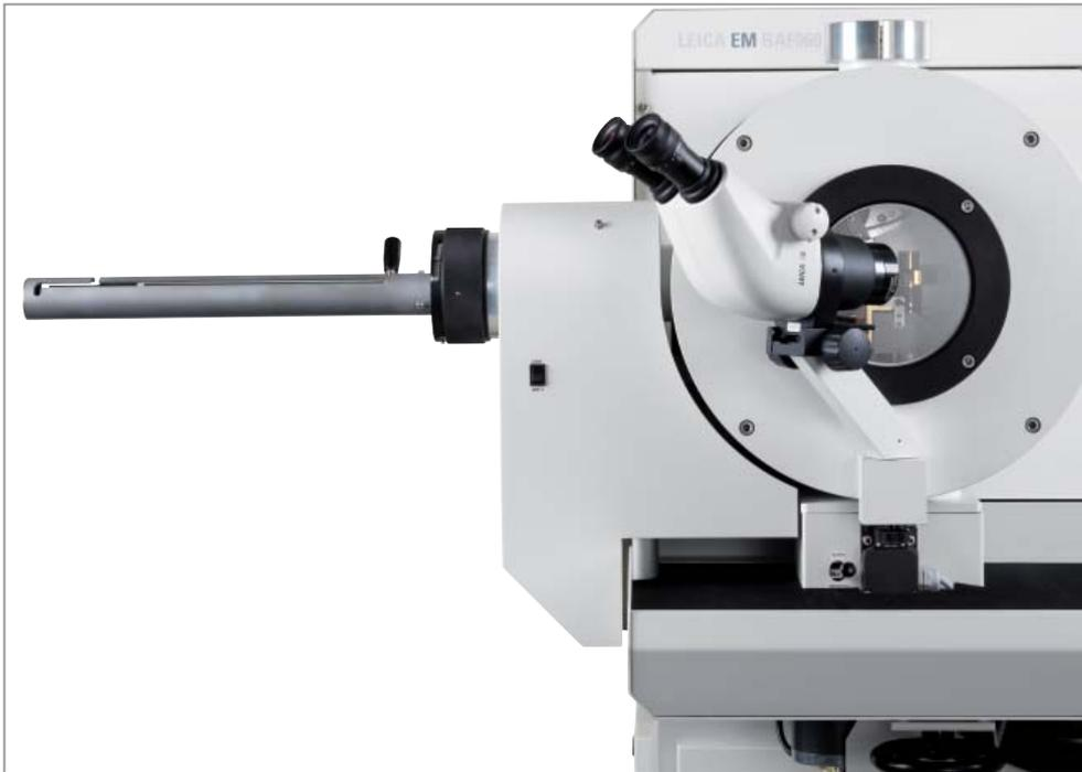
Load-lock transfer rod for quick and easy **sample exchange**.
