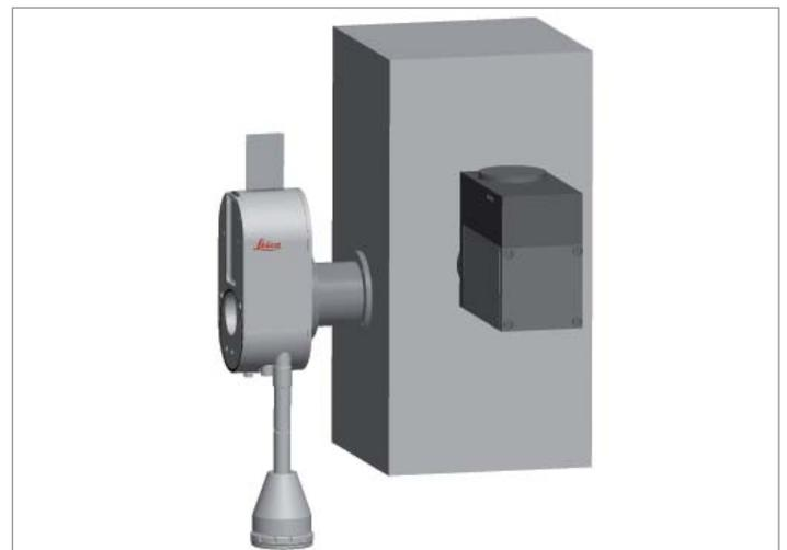
EM VCT100 docking station and cryo Dewar on an analysis instrument.
