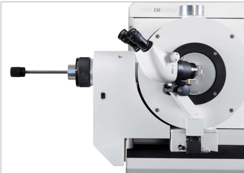
Load-lock transfer rod for a one button operational **exchange of the electron beam gun and coating material**. The process is extremely easy and quick.
