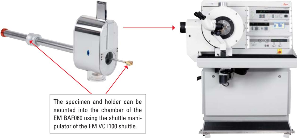
The specimen can then be fractured, etched and coated using the multiple features of the Leica EM BAF060.
