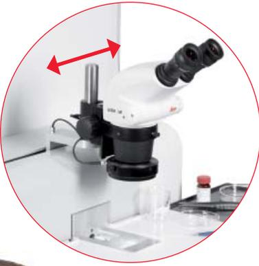
The integrated stereomicroscope can slide left and right allowing better sample viewing and access during preparation and processing. It comes complete with adjustable LED illumination.
