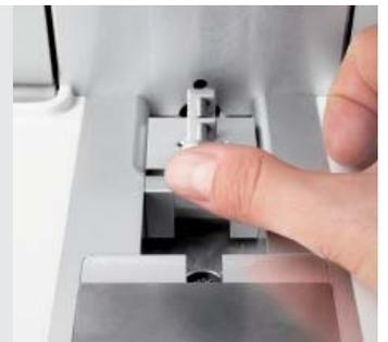
After cryofixation, the frozen sample is automatically released into the LN<sub>2</sub> Dewar.
