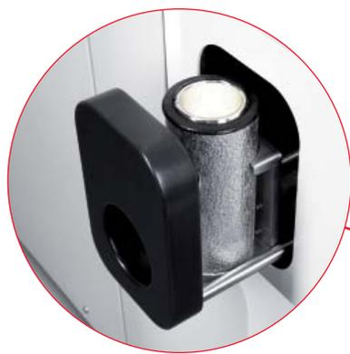
The vitrified sample is automatically released into a conveniently located LN<sub>2</sub>-filled Dewar. The sample stays well frozen at all times.
