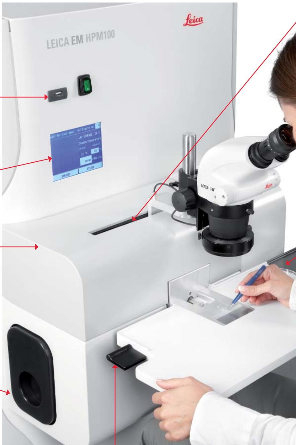
Well-positioned cartridge lever for quick manoeuvring of the sample cartridge.
