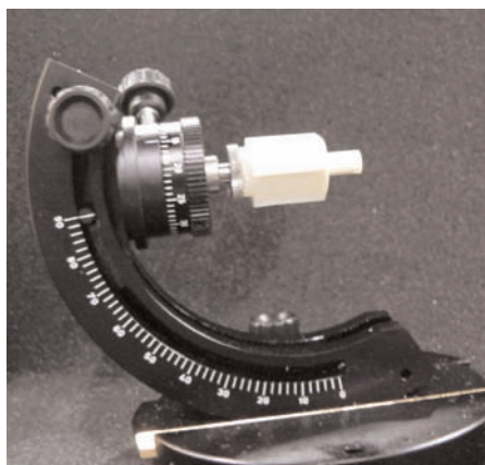
IBIS bullet mount, positioned on the push-in cartridge case mount (cat. #11581085)
