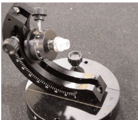
10mm/40 cal cartridge case push-in mount (cat. #11581085) positioned in universal specimen mount.
