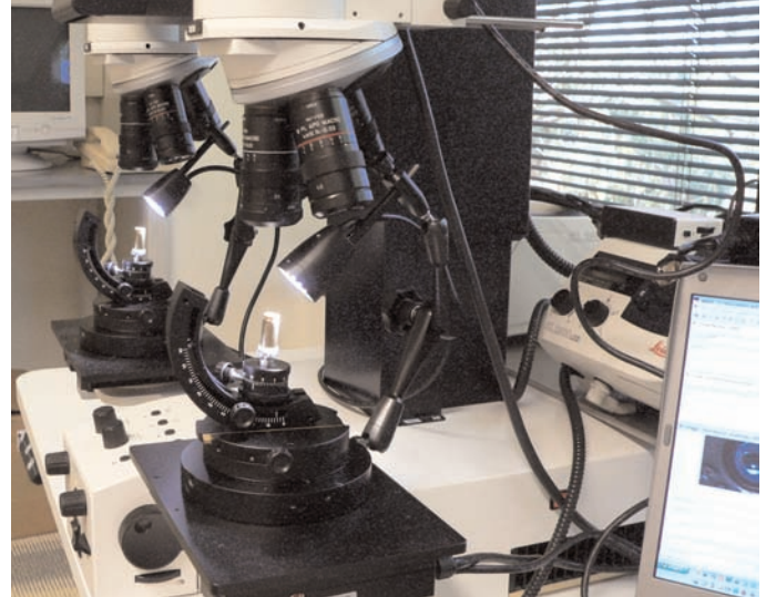
Figure 1: Spot LED mounted on a comparison microscope
