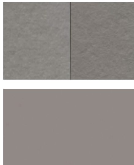
Figure 4. Blank live image before (top), and after (bottom) shading correction is applied.
