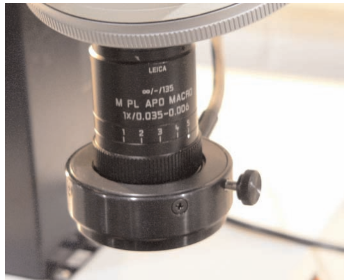
Figure 2: LED ring light mounted on macro objective
