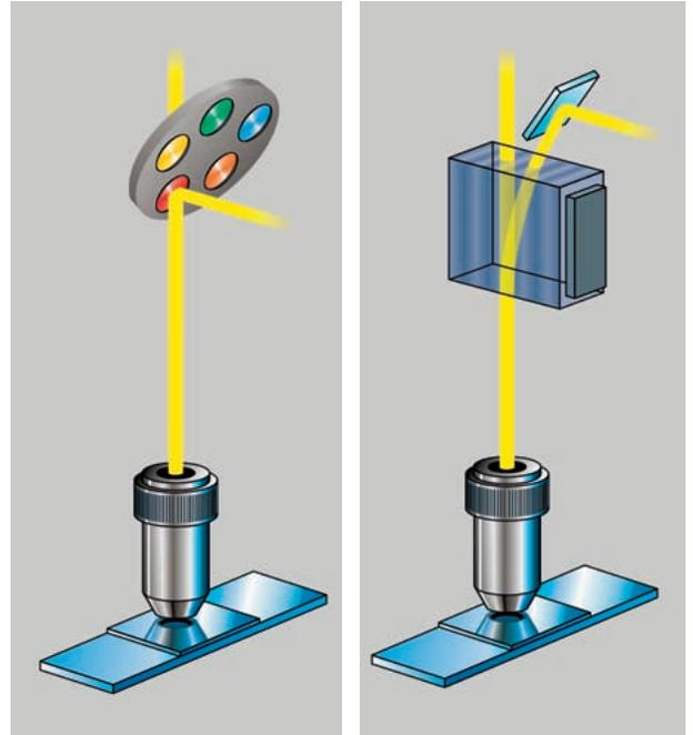
Left: conventional beam splitting by dichroic mirrors requires many optical elements with fixed properties.
