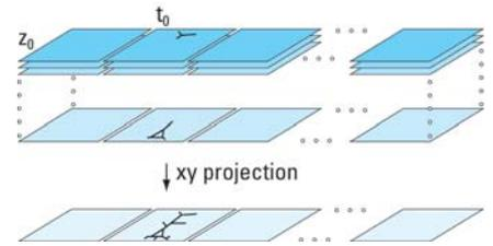
XYZ-Scan Module: Time series at different focal positions, stimulus ( $t_0$ ) is always delivered before the same frame of each time series
