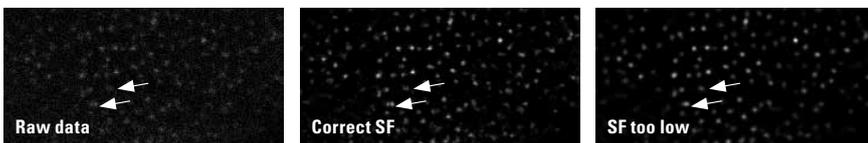
**Fig. 4** Effect on image quality with the saturation factor set too low. Arrows indicate spots that show the loss of obvious substructures, which can be clearly identified in the raw data.
