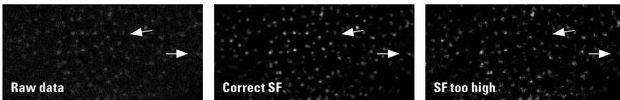
**Fig. 3** Effect on image quality with the saturation factor set too high. Arrows indicate possible artifacts (noise amplification and excessive granulation and contrasting of structures).
