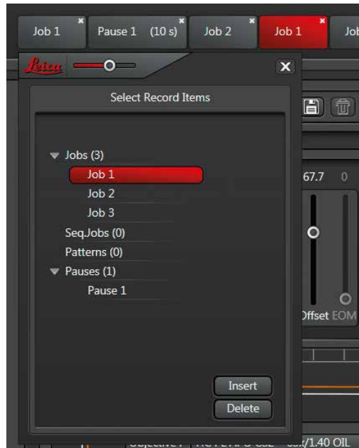
Figure 10 Example for a reference: Job 1 in the list is the reference of both Job 1 records in the time line.
