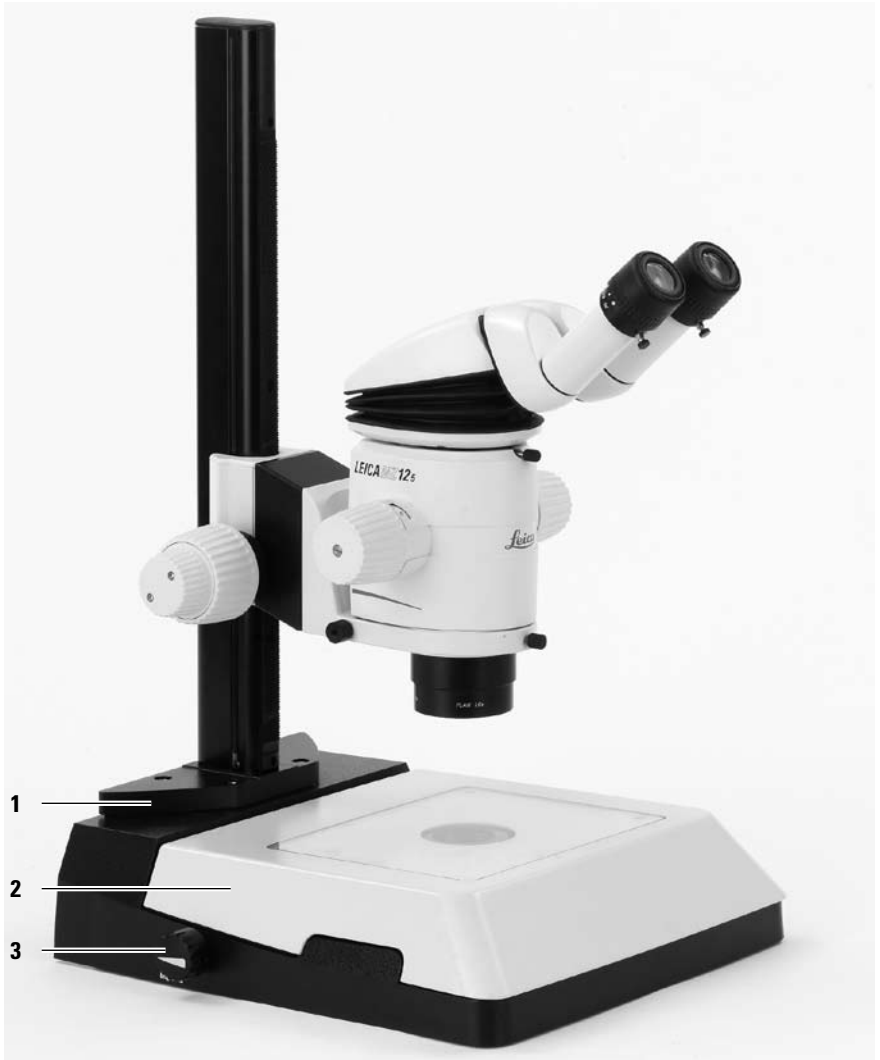
Fig. 1 Leica MZ16 with ErgoTube™, coarse/ fine drive, TL BDFD transmitted-light base, standard stage and 4xslides
