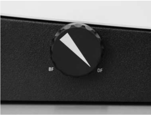
Fig. 4 Button to toggle between bright field/ dark field (here: Button in dark field position)
