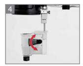
Look through the eyepieces and switch to maximum magnification. Use the focusing lever on the prism block for fine focus.
