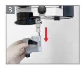
Firmly hold the prism block while carefully lowering the Leica RUV800.
