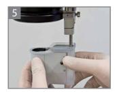
Pull the sterilizable cover over the Leica RUV800.
