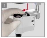
Press the clip on the suspension downwards and pull the Leica RUV800 out of the holder.
