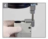
Push the prism block into the holder on the suspension so that it clicks into place.
