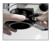
Fasten the adapter to the front threads using the two screws.
