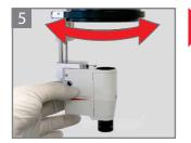
Rotate the Leica RUV800 into the desired position.
