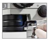
Tighten the screw on the suspension.
