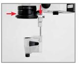
Working distance WD200: The WD designation of the objective must agree with the laser inscription on the suspension.
