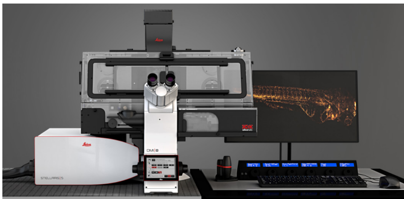
Fig. 23| STELLARIS 5 DLS system with a transparent cage incubator to keep the temperature constant during long acquisitions.
