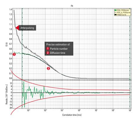
FCS curve acquired with HyD SMD (green) and Avalanche photodiode (grey). Sample: 10 nM Alexa 488 in water. The plateau in the microseconds area allows precise estimation of particle concentration. The residuum (green) indicates optimal fit quality. Particle number: n = 2.3, Diffusion time:  $\tau = 24 \ \mu s$ .
